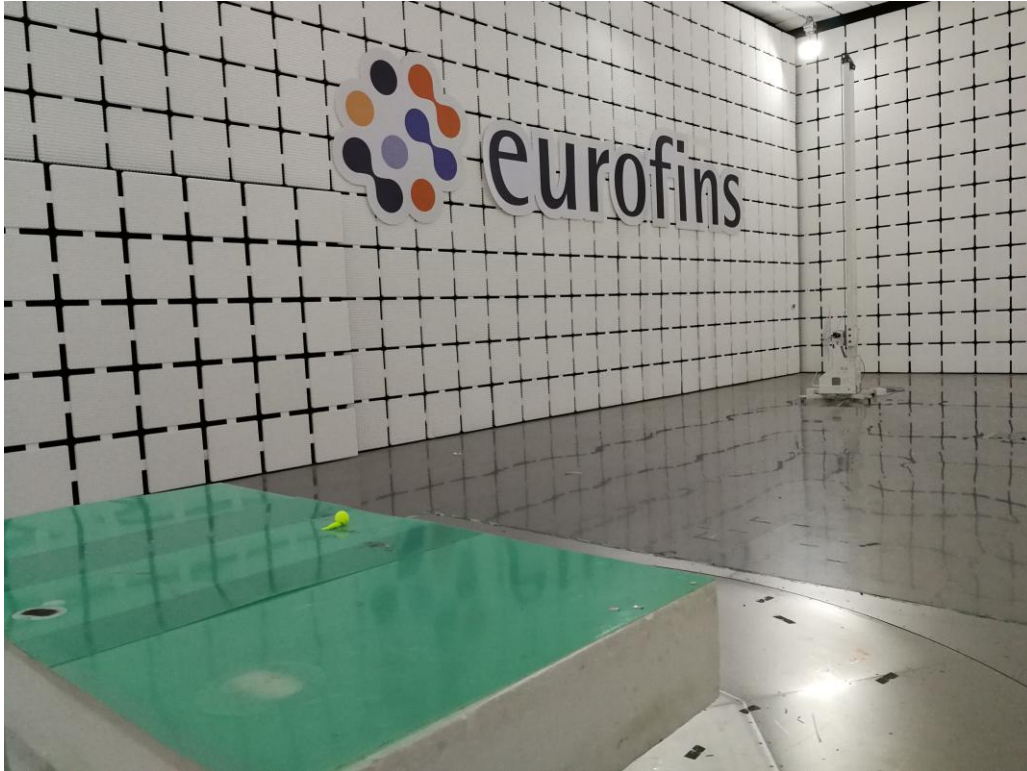
Picture 2 Radiated Emission Test Setup
